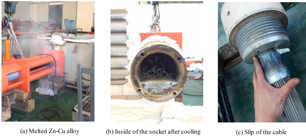
Fig. 5. Failure of Hot-Cast Anchor Socket Specimens.
